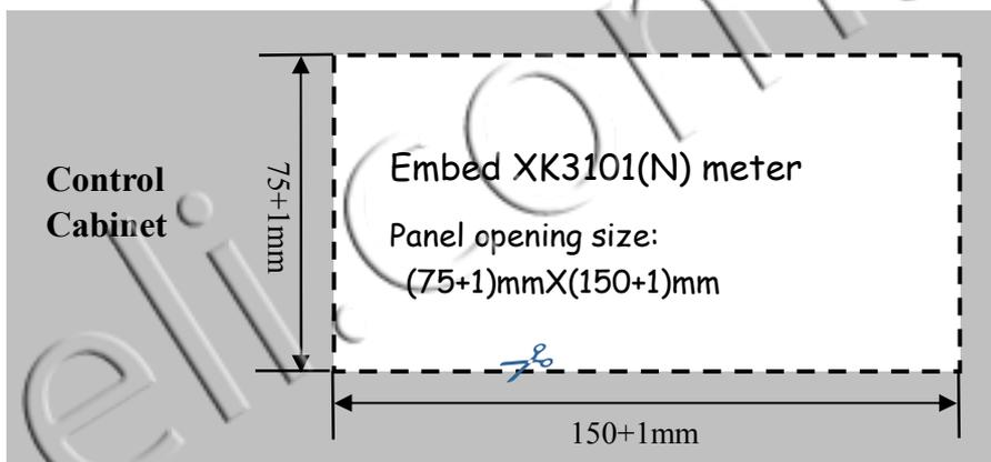
Before installation, mandril of both sides of housing should be removed firstly, and then put into the cabinet from the front side. The two mandrils are fixed to both sides of indicator tightly to guarantee the firm installation. The depth of cabinet is not less than 180mm, easy for wire connection.
