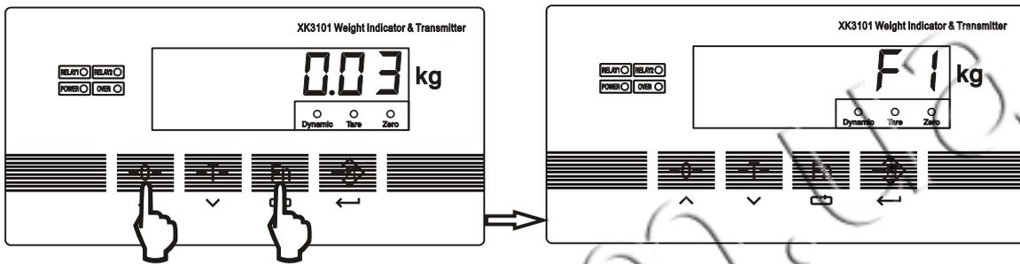
2. Press **【PT】** button, indicator shows “CAL X”, “X” means the previous calibration method.
