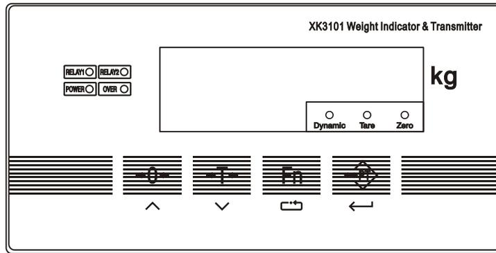
The indicator has four buttons on display Panel, used for all operations and parameters set-up for indicator.
